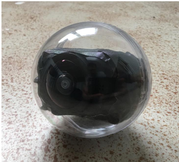
*Figure 1: The 360° camera encased in the new housing.*
